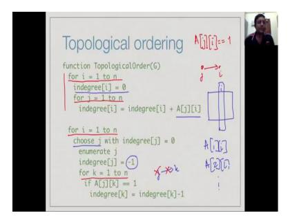
So, let us look at some pseudo code for the algorithm which we just executed by DAG. So, in this particular algorithm we first start by computing the in degree, so in order to compute the in degree, we need to find out how many for a vertex i we need to find out how many j satisfy the property that A j i is equal to 1, because this corresponds to an edge from j to i. So, when an adjacency matrix this corresponds to looking at a column containing line.
