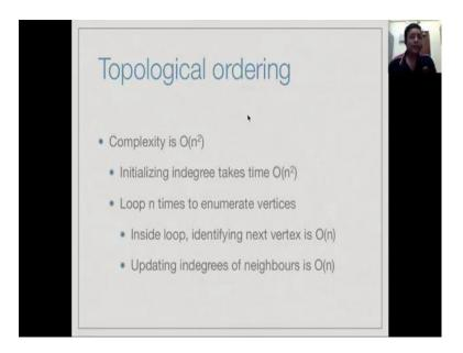
So, what is the complexity of the algorithm is fairly easy to see that for this adjacency matrix or presents it is n square, as we saw initializing the in degree itself takes time n square ((Refer Time: 16:01)). Because, we have one outer loop from 1 to n and then for
